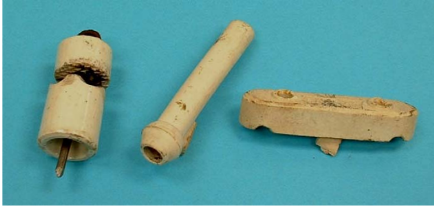
Fig. 2 – Old Knob, Tube, and Cleat
