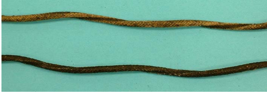
Fig. 15 – Old Conductor of Natural Gray (top) and Black (bottom) Cotton Braid
