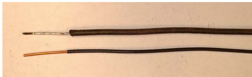
Fig. 5 – Older Tinned Rubber Wire (top) and Newer 90°C Wire (bottom)
